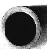
FIG. 4 Photomicrographs of Tube Ends after 1 min of ECM Solution flow rate of 0.085 l/min for two concentrations, 50 g/l A, B, C and 250 g/l D, E, F, of NaCl A, D, NaClO 3 B, E and Na 2 Cr 2 O 7 (C, F at an applied voltage of 10 V).
